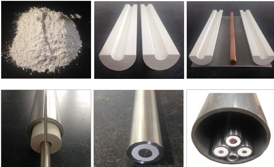
Figure 1 – Steps in the fabrication process for Salamander heaters are shown above. Magnesium oxide powder (electrical insulation material) is formed into grooved blocks. The central electrical conductor rod is added. The outer stainless-steel sheath is formed around the blocks to provide corrosion resistance. The assembly is drawn to the final length. Multiple conductors and instrumentation tube are pulled into carrier pipe, ready to be assembled on a reel and shipped to the site.
